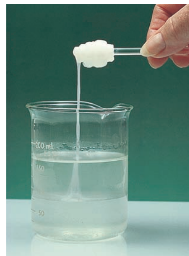
Figure 15.26 The formation of nylon-66. Nylons are formed industrially by the reaction of diamine and diacid monomers. In this laboratory demonstration, the six-C diacid chloride, which is more reactive than the diacid, is used as one monomer; the polyamide forms between the two liquid phases.
